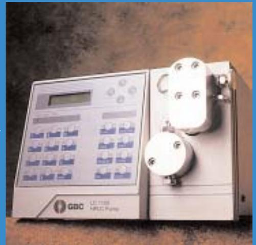
GBC 1100 Series Solvent Delivery Modules are designed specifically for the analyst. Free-floating dual in-series pistons, with variable volume delivery, guarantee reproducible flows with low piston-seal wear. This means accurate quantitative determinations.
