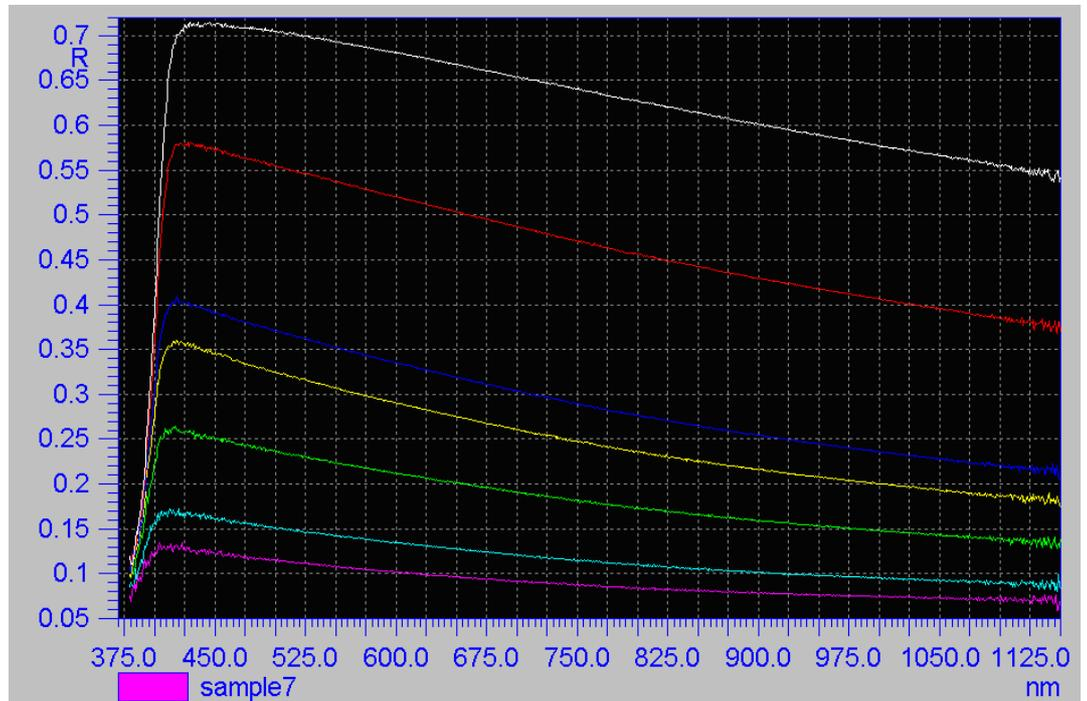
**Figure 3: Actual Military Cloth designed to camouflage in NIR region and at key laser wavelengths.**
