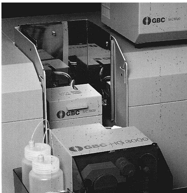
**Figure 5:** Installation of the mercury concentrator in a GBC 906 Elite AA, showing the HG3000 vapour generator, the MC3000 workhead and separate controller/power supply.
